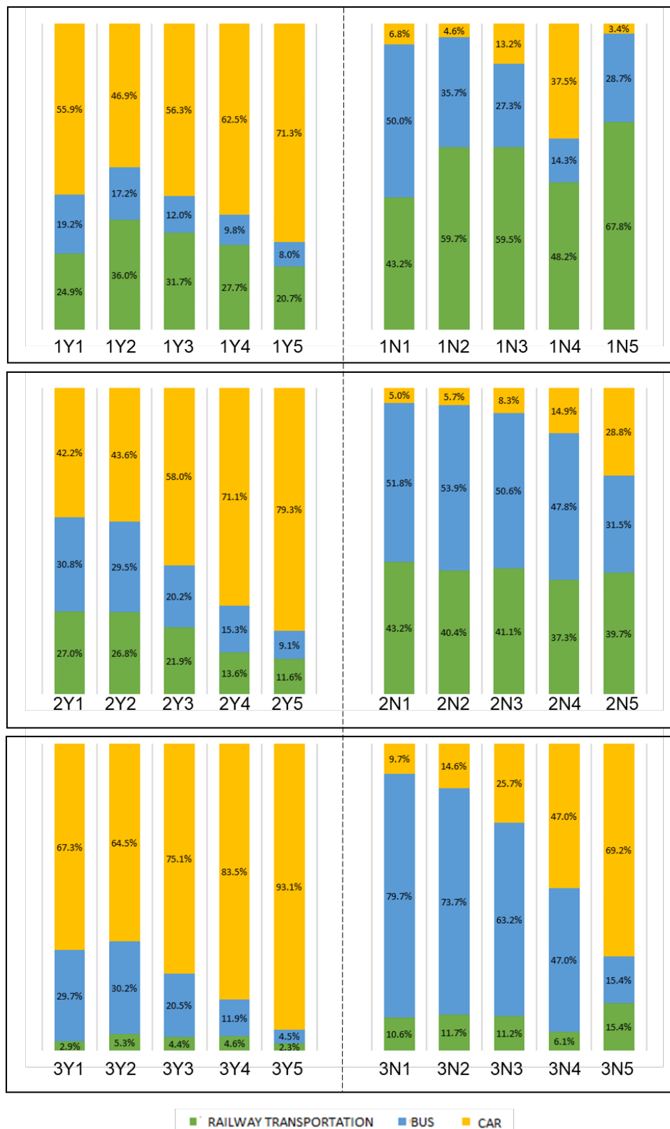
Figure 5. Modal share considering the car ownership (Y – yes or N – no) and the household income level (1 to 5) for (1) trips with both the origin and the destination closer than 1 km from a railway station, (2) trips with only the origin or the destination closer than 1 km from a station, and (3) trips with both the origin and the destination farther than 1 km from a station
